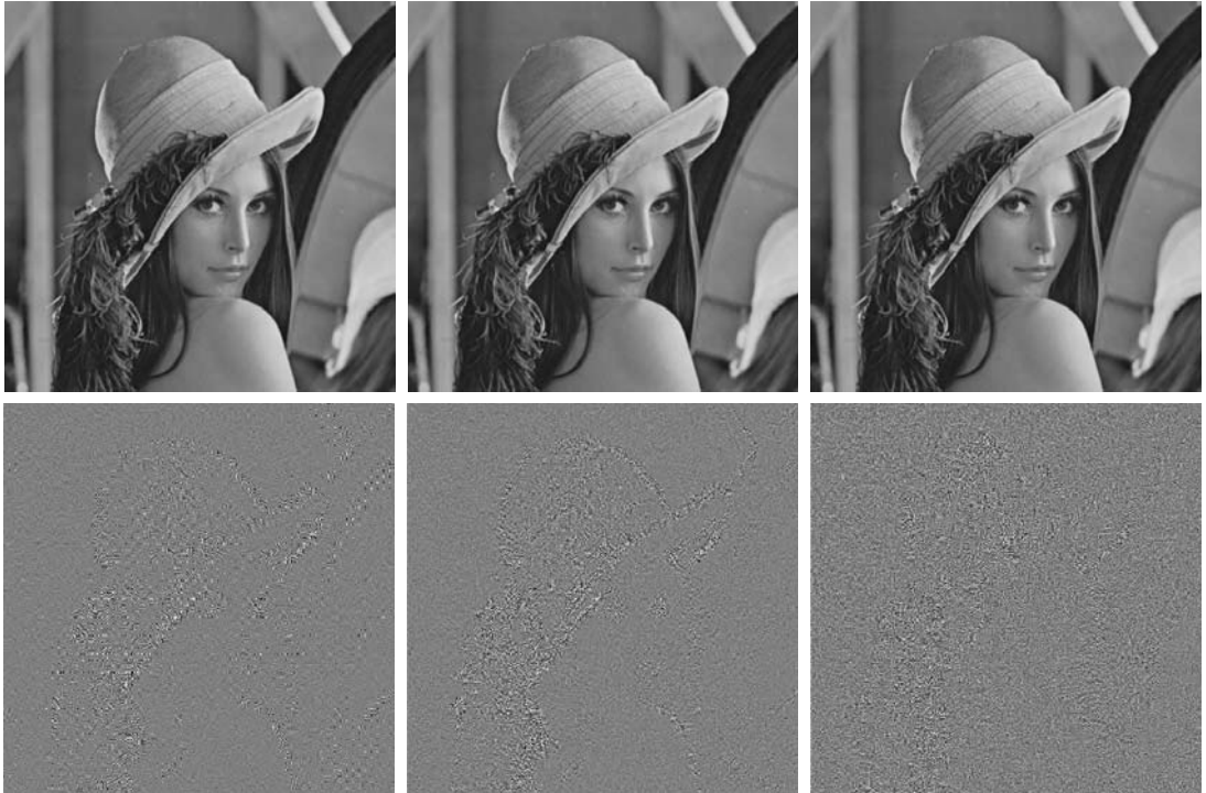
FIGURE 8.24 Approximations of Fig. 8.9(a) using the (a) Fourier, (b) Walsh-Hadamard, and (c) cosine transforms, together with the corresponding scaled error images in (d)–(f).
