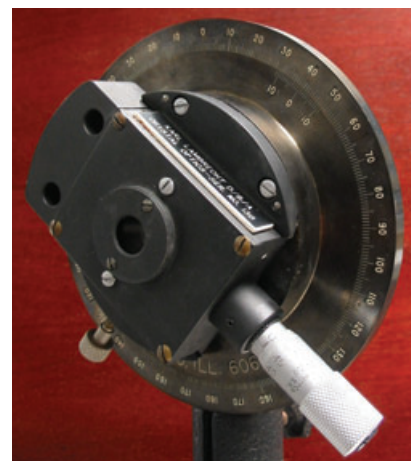
Babinet-Soleil compensator manufactured by Karl Lambrecht Corp. of Chicago, Illinois, USA, and obtained by the author in ca. 1966. This device incorporates two crystal quartz wedges and a flat quartz plate mounted in a precision azimuth mount. At \lambda = 633 \text{ nm} , the least Retardation reading is 0.0065\lambda , and range is 6\lambda . Photo by G. L. Cloud at Michigan State University, 2011.
