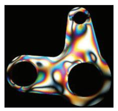
Stress analysis of a metal bellcrank using a photoelastic coating. This procedure facilitates optimization of the component to improve strength-to-weight ratio. Linear polarization was used for this study, so an isoclinic fringe appears with the isochromatics. Can you identify its paths? Photo courtesy of Dr. Eddie O'Brien, Past President of SEM, Consultant—Aircraft Technical Solutions, Ltd.
