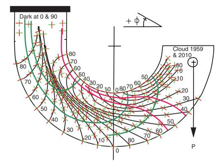
Detailed steps to construct a stress trajectory pattern are given below along with some tricks to ease the process and some traps to avoid:
