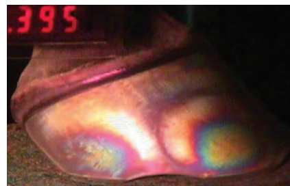
An isochromatic fringe pattern from photoelastic coating experiments to determine effects on the stress state in equine hooves resulting from different trim practices by farriers. Crippling diseases such as laminitis are related to hoof stress. Photo courtesy of Dr. Loic Dejardin, DVM, of the College of Veterinary Medicine, Michigan State University.
