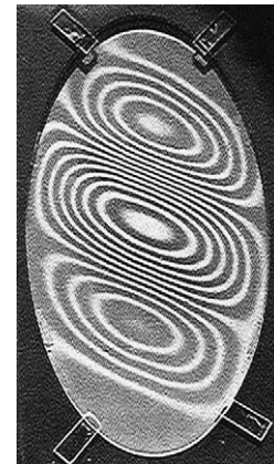
Shadow moiré pattern showing buckling mode of elliptical graphite/epoxy [45^\circ]_8 composite panel with clamped edges. From Singhatanadgid, P., and Tuttle, M., “Buckling of Elliptical Anisotropic Plates Subjected to Biaxial Loading,” Proceedings of 2000 IX SEM International Congress on Experimental Mechanics. Photo courtesy of Dr. Mark Tuttle, Chair of Mechanical Engineering, University of Washington.
