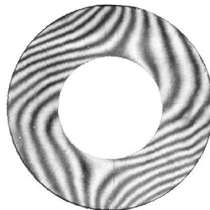
Geometric moiré pattern for a ring in diametral compression obtained during a student lab demonstration using 500 lines/inch gratings with a transparent plastic specimen. Pitch mismatch, rotation, and strain affect the pattern. Photo by Gary Cloud, ca. 1970.
