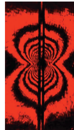
Micro-photoelasticity interferogram showing stress state near a single glass fiber embedded in epoxy matrix after fiber rupture. Courtesy of Dr. Pedro Herrera-Franco† and Dr. L.T. Drzal‡
